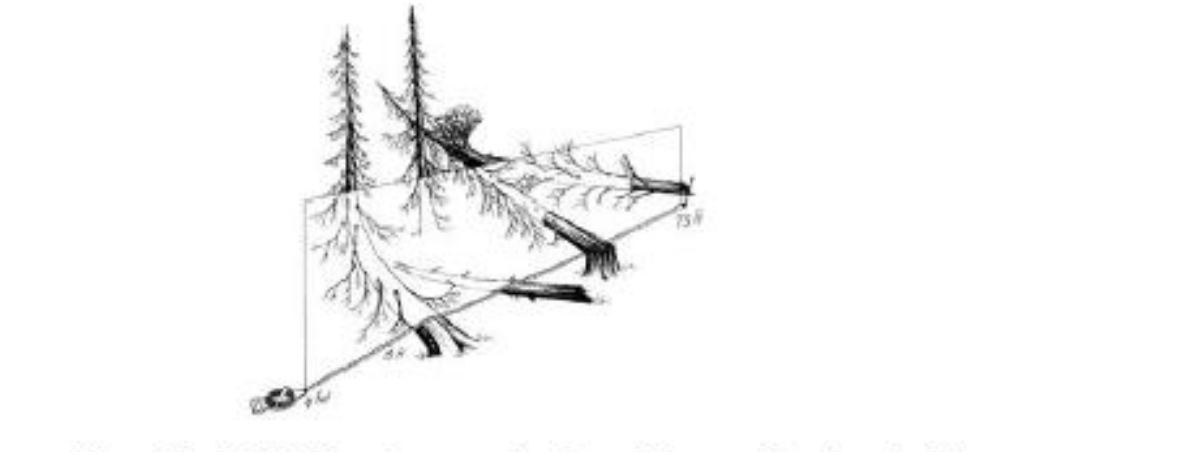
Figure 27: All of the pieces crossing through the sampling plane of coarse woody debris (1000-hr fuels) that would be measured in the line intercept fuels sampling method.
