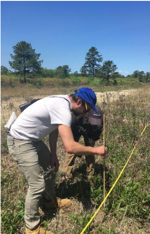
Figure 13: Transect line for line-point intercept sampling, laid flush to the ground.
